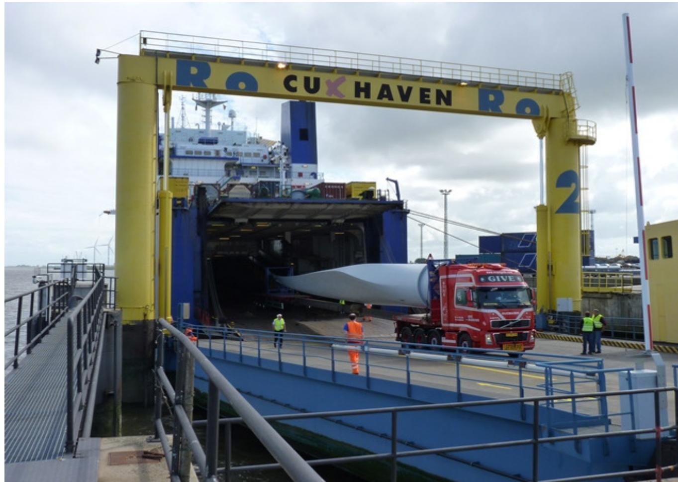
Load Option 5: Rolling by use of RoRo-ramp – up to 350 t cargo weight
